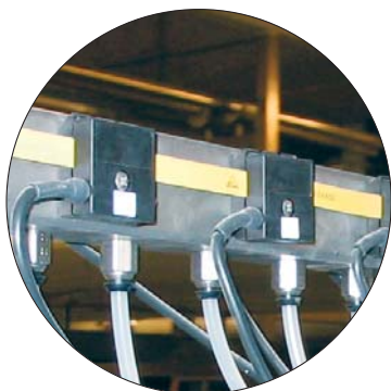
AS-Interface vampire contact for the control module e BUS
